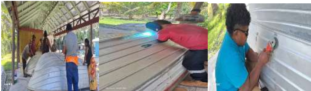
Figure 5 Aluminium boat repair (Niutao)
