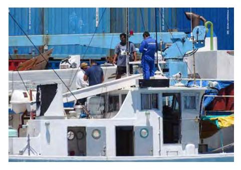
Figure 32: Fisheries mechanics and Furuno expert installing the new echo sounder on RV Manaui
