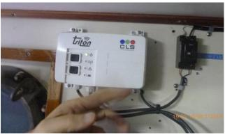
Figure 24: Isolation switch on a MTU on a foreign longliner
