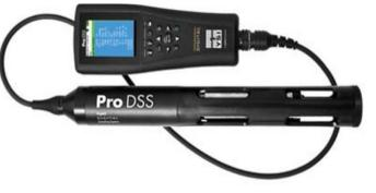
*Figure 30:* Hand-held water quality meter and probes purchased by TFD for water quality monitoring.
