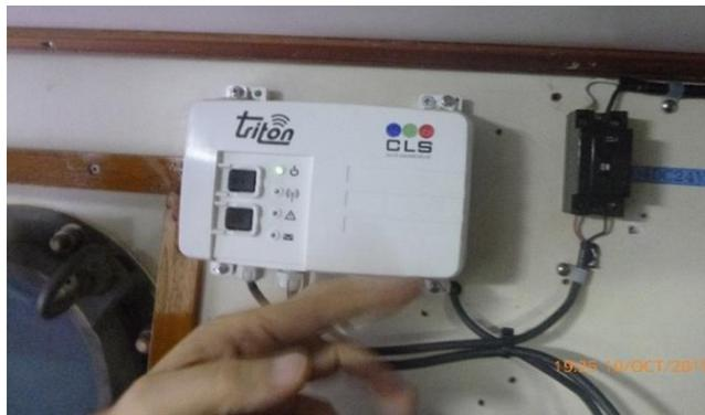
Figure 24: Isolation switch on a MTU on a foreign longliner
