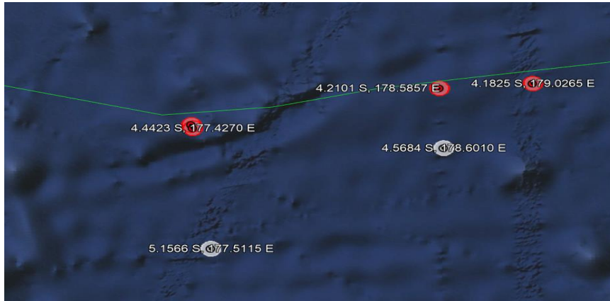
Figure 35: satellite scan results correlated to VMS data & AIS. Grey means ok & red means unidentified or unknown and could potentially be an IUU vessel
