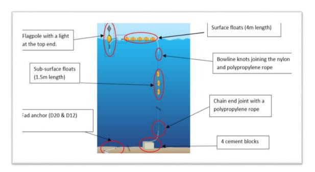
Figure 33: Lizard FAD Structure and design deployed in Nui
