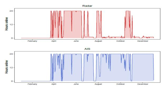
Figure 26: Hours per day that the M2 radar system and AIS were functional.
