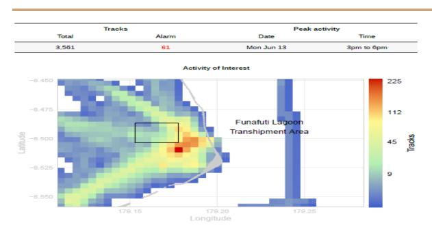
Figure 25: The map shows tracks detected by radar and the Automatic Identification System (AIS) with an average speed of fewer than 6 knots or triggered a preset alarm zone.
