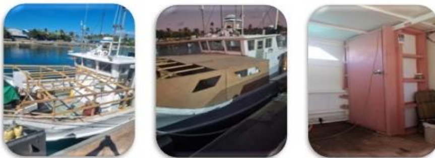
Figure 16: Manau I new passenger shelter
